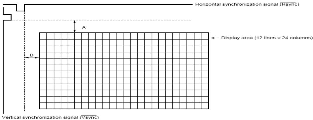
A:  $9H \text{ (line)} \times (2^4V_4 + 2^3V_3 + 2^2V_2 + 2^1V_1 + 2^0V_0)$
